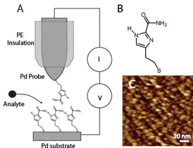
**Figure 1.** Recognition tunneling with Pd electrodes. (A) A Pd covered Si wafer is functionalized with a monolayer of an imidazole-carboxamide molecule (B) as is the end of an electrochemically etched Pd wire. The wire is insulated with polyethylene, leaving a fraction of a square micron of exposed area. The junction is submerged in buffered aqueous electrolyte containing analyte molecules that diffuse into the tunnel junction. (C) STM image of a Pd coated substrate showing 10 nm grains.
